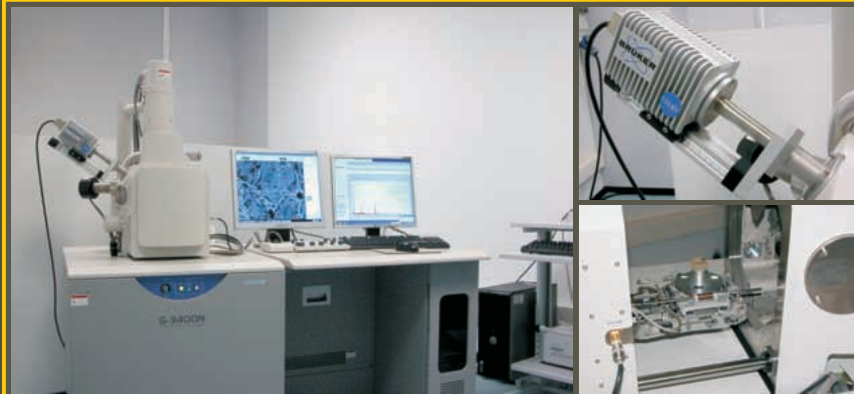
SEM Hitachi S400n and Bruker Xflash 4010 detector used in the study. Photo.: G-Vuelta
